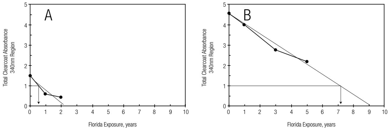
*Figure 2. Decrease in total clearcoat absorbance in the 340 nm region as a function of Florida exposure*
