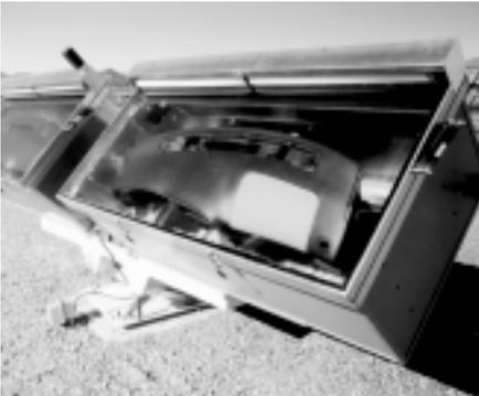
The TNR method will replace SASR (Seasonally Adjusted Solar Radiation) for all GM natural weathering tests of interior automotive materials that require exposure in high temperature limited test fixtures. AWSG refers to these fixtures as “IP/DP Boxes.”
