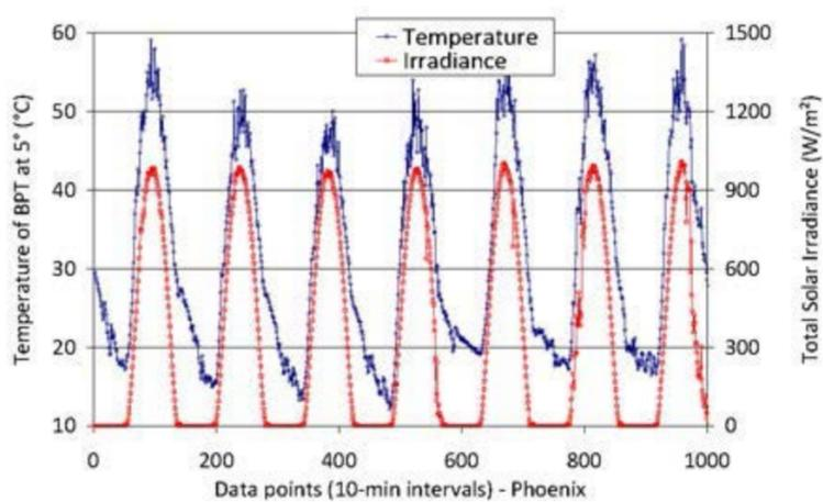
Figure 1 - Temperature and irradiance changes of a typical week in Phoenix, Arizona
