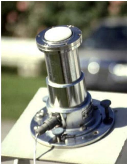
*Total Ultraviolet Radiometer (TUV)*
