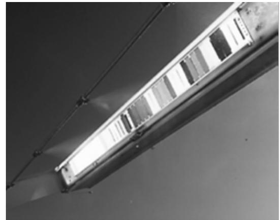
**Figure 5:** EMMAQUA® water sprays provide thermal shock or night time dew wetting.
