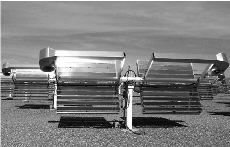
**Figure 4:** EMMAQUA® solar concentrator for accelerated weather testing.
