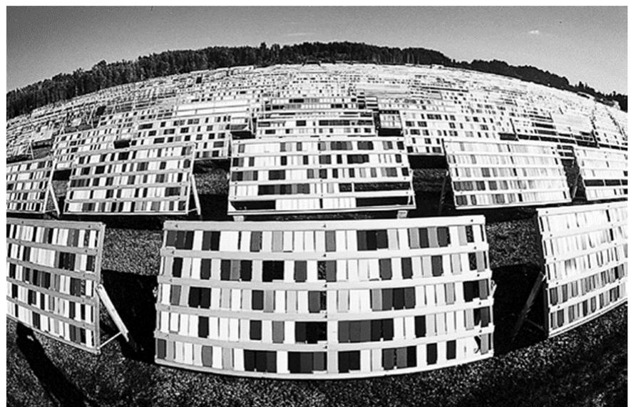
**Figure 3:** Fisheye view of some of the "test fences" at South Florida Test Service near Miami, the world's largest exposure facility and primary coatings benchmark climate.
