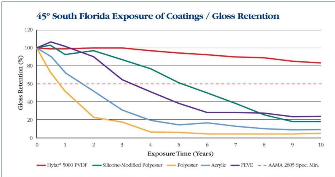
**Figure 2.** Plot of gloss retention (%) of architectural coatings during weathering exposure. Courtesy Solvay. <https://www.solvay.us/en/print.html?tcmURI=tcm:182-228910> accessed 2018-05-17.
