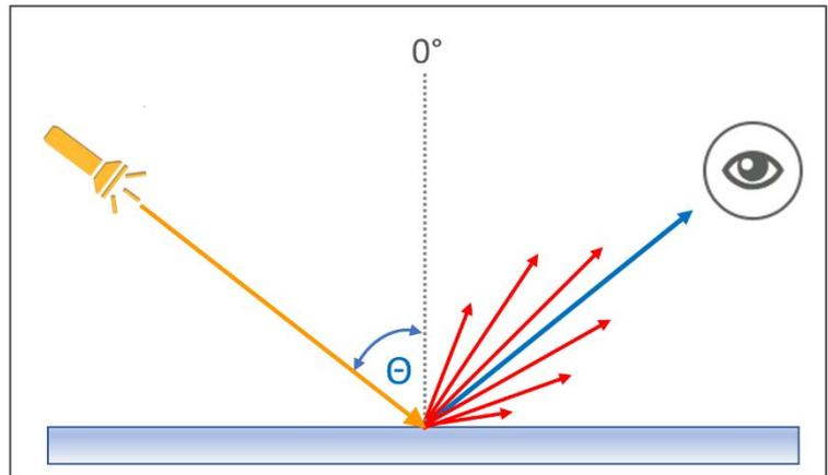
**Figure 1.** Gloss consists of incident light of known intensity (yellow line) at angle Theta ( $\Theta$ ), specular reflection at the same angle but lower intensity (blue) and scattered light (red). Typical angles are 20°, 60° and 85°.
