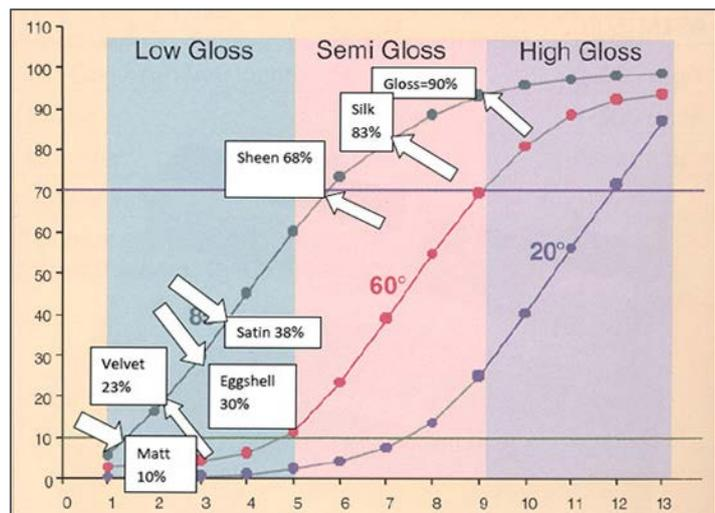
**Figure 3:** Plot of gloss for 13 coatings using 60° angle.
